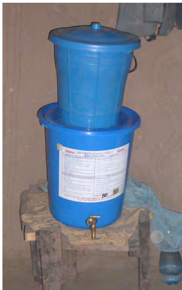
Figure 1. Fluoride removal household filter in the main house of a rural family in the Ethiopian Rift Valley (Images by Lars Osterwalder, Eawag).
