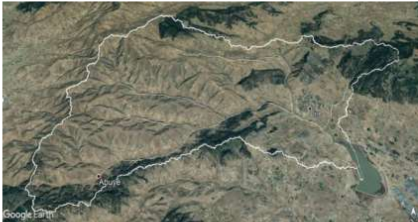
Figure 5.1 Delineation of Dire Dam Water Catchment
