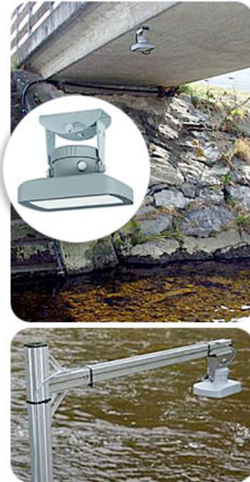
Figure 53 Typical radar (RLS OTT) - in air (look down) water level sensor
