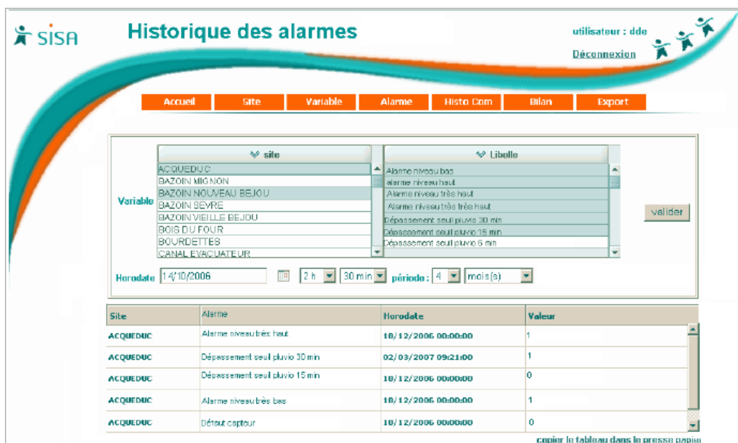
Figure 64 supervision software : Alarms screen examples
